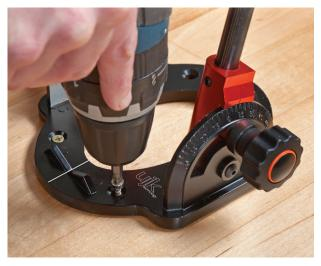
• The UJK drill guide can be fixed in postion using the four countersink holes in the drill guides base, see picture above.
