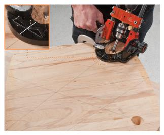
• Drilling holes at set angles, see top picture. Using the site lines to align the UJK drill guide before drilling, see picture above.
