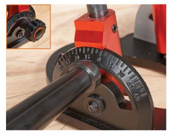
• The Quadrents on both sides of the base allows the assembly to be tilted + or - 60° and clamped in place with the clamping knob.
