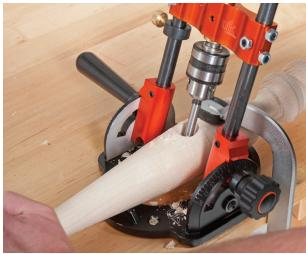
• The UJK drill guide can be used to drill rounded material, ideal for chair legs, see pictures above.
