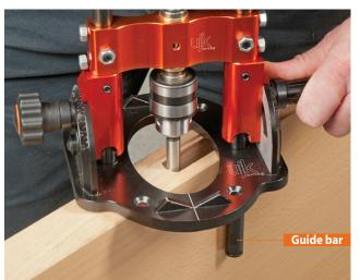
• The steel guide-bars can be set to protrude through the base. When drilling a lock mortice, engaging the protruding bars on either side of the door automatically self-centres the guide, see pictures above.
