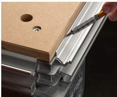
Close any gap visible between the extrusion and table top.
