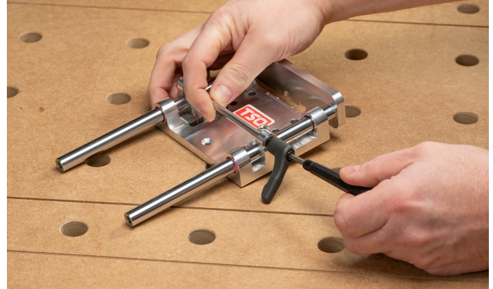
Step 1. Using a Torx T20 driver, unscrew the Lever completely. Hold the clamp shaft steady with your free hand.
