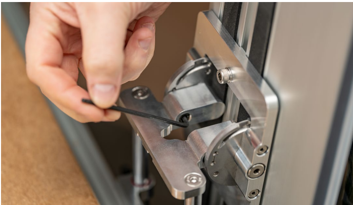
Step 2. Using the 3 mm hex key, adjust the two black hex screws on the inside of the hinge—clockwise to increase positive stop strength, counterclockwise to reduce it.
