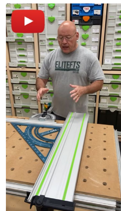
Brian Sedgeley walks through squaring the Festool MFT/3 using the back fence adjustments. Watch the video.
