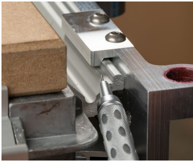
Example of hook set correctly—inward for MFT/3, always facing down.
