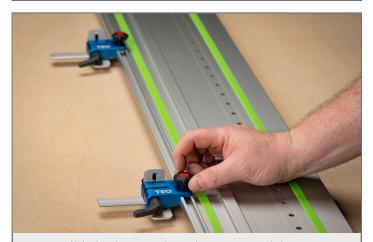
**Step 3.** Slide both Gages into the top T-track in your guide rail, and tighten the top comfort-grip knob to secure them in place. Keep the lever arms loose so the Gage Bars can slide back and forth.
