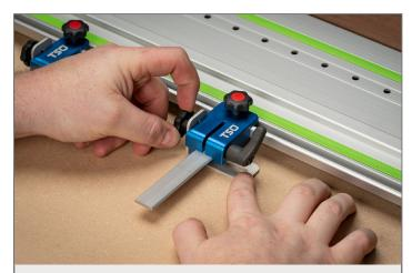
**Step 12.** To set the foot height of the Gage Bar, release the side-mounted comfort grip knob and drop the foot to the work surface. Tighten the knob to secure the foot in place. Repeat for the other Gage Bar and Support Feet, if used.
