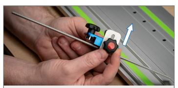
**Step 2.** Before installing the Gages, ensure their adjustable feet are fully retracted. Repeat for the other Gage and Support Feet, if used.
