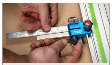
**Step 7.** Release the clamping lever and pull out the Gage Bar to your desired cut width. Using a precision rule, align your desired cut width on the rule to your pencil mark. (Above, we're showing a 1" cut.) Once aligned, tighten the clamping lever to fix the Gage Bar in place. Repeat for the other Gage Bar. *Skip to Step 11*.
