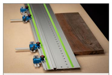
**Step 11.** Slide on additional Guide Rail Support Feet as needed. Here, they are shown supporting track saw lead-in and lead-out, but they can also be helpful in preventing guide rail deflection between the Gage Bars for longer cuts.
