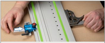
**Step 9.** Keeping the face of the Combination Square against the splinterguard, push in the Gage Bar until it contacts the blade of the Combination Square.
