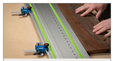
**Step 4.** Slide your workpiece snugly against the guide rail splinterguard.
