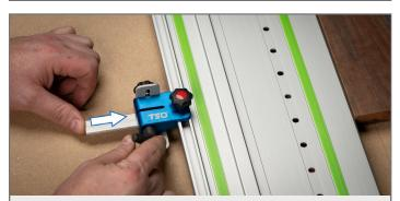
**Step 5.** Push the Gage Bar underneath the guide rail until it comes in contact with the workpiece. Rotate the clamping lever clockwise to secure it. Repeat for the other Gage Bar.
