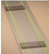
**Step 1.** Elevate your guide rail with thin strips (roughly 3/8" in thickness) located at the far ends. Alternatively, if installing onto a Festool MFT/3 or other worktop with a means to elevate and fix the guide rail in place, position the guide rail about 3/8" above the worktop.
