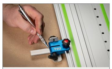
**Step 6.** Mark the "Zero Line" on the Gage Bar, where the bar meets the body, using a sharp pencil or fine mechanical pencil.
