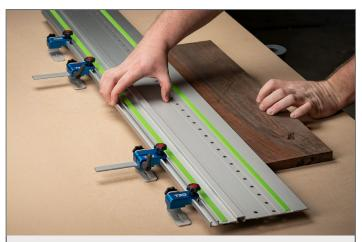
**Step 13.** With the Narrow Stock Pro components installed and calibrated to your desired cut width, place your Guide Rail on top of your workpiece and slide right until both Gage Bars make contact with your workpiece edge. You're ready to make the cut!
