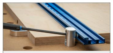
**Step 3.** Slide the Fence Extrusion through the torpedo nuts on both Fence Dogs and, once in position, tighten both Fence Dogs screws using an M5 Hex Driver.
