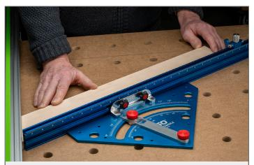
**Step 3.** To adjust Fence angle, loosen the two red knobs on the MTR-X protractor and rotate the Fence and Triangle Assembly to any angle. Secure in place by re-tightening both red knobs on the MTR-X protractor.
