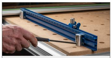
**Step 5.** Gently tighten both Fence Dogs screws using an M5 Hex Driver.
