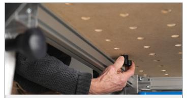
**Step 2. IMPORTANT:** Always clamp both Fence Dogs securely from underneath the table using **M8 SpeedKnobs** or equivalent M8 clamping knobs. Failure to properly secure the Fence Dogs may result in product damage or unsafe operation. (Clamping knobs sold separately.)
