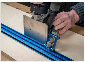
**Step 4.** Optionally, the included Flip-Stop can be used as a router or Domino stop.
