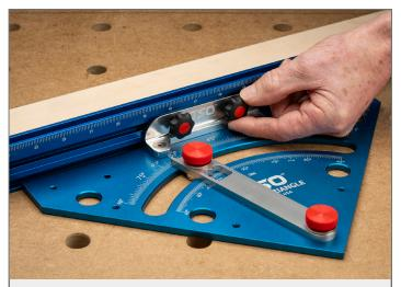
**Step 2.** Install the protractor assembly included with the <u>MTR-X Precision Triangle</u> and secure to table at the desired angle. Slide Fence Extrusion through the two Square Nuts on the Connector. With the Fence positioned as desired, tighten the two comfort grip knobs on the Connector. Tighten the two red knobs on the MTR-X protractor.
