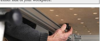
**Step 2.** Optionally, clamp both Fence Dogs from underneath the table, using M8 SpeedKnobs or a similar M8 clamping knob. (Clamping knobs sold separately.)
