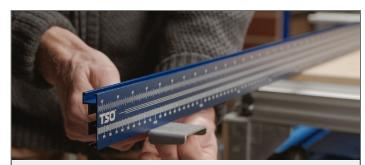
**Step 5.** Attach the **Stock Support & Stop Bracket** (sold separately) to the bottom T-slot of the Fence Extrusion.
