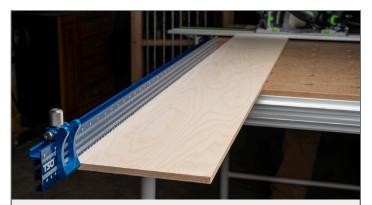
**Step 6.** Slide the Flip-Stop onto the Fence Extrusion, using the upper T-slot. Position to desired cut length, and tighten the knurled knob to fix in position.
