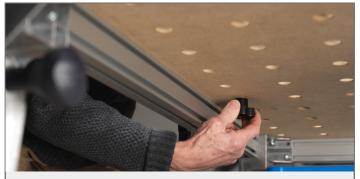
**Step 2.** Optionally, clamp both Fence Dogs from underneath the table, using M8 SpeedKnobs or a similar M8 clamping knob. (Clamping knobs sold separately.)
