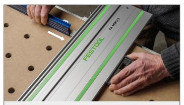
**Step 4.** Using a Combination Square set to 7-7/8" (200mm), slide it under the Guide Rail until the square's head touches the splinterguard. Then, slide the Fence Extrusion until it makes contact with the end of the Combination Square blade. As an alternative to a Combination Square, you can use a scrap piece of wood or panel cut to 7-7/8" long.
