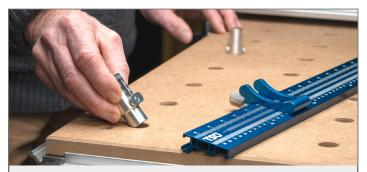
**Step 1.** With your guide rail installed and flat on your worktop, insert both Fence Dogs corresponding to your preferred fence location.
