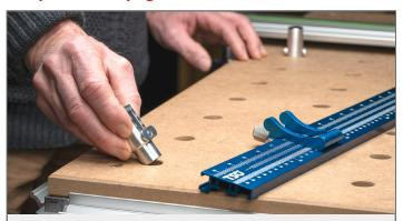
**Step 1.** With your guide rail installed and flat on your worktop, choose your preferred fence location. Typically, to maximize your table's cutting envelope, this will be the furthest row of dog holes. Space each Fence Dog as far apart as possible.
