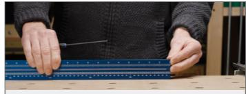
**Step 3.** Slide the Fence Extrusion through the torpedo nuts on both Fence Dogs.
