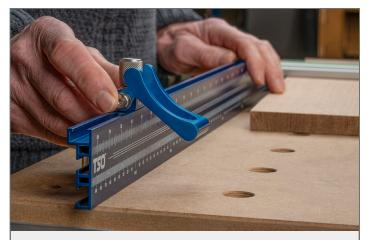
**Step 6.** Slide the FlipStop onto the Fence Extrusion, using the upper T-slot. Position to desired cut length, and tighten the knurled knob to fix in position.
