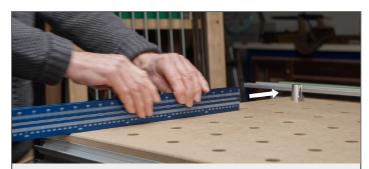
**Step 3.** Slide the Fence Extrusion through the Torpedo Nut on both Fence Dogs, using the bottom (large) T-slot on the back of the Fence Extrusion. Position the Fence Extrusion so that it is approximately 3/8" (10mm) from the track saw guide rail. *Do not tighten Fence Dogs yet*.
