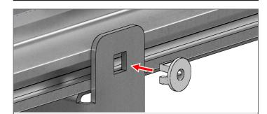
**Step 13.** Insert four *Plastic Inserts* (with the snap "teeth" facing up and down) into the square holes in the *Bracket* and into the T-slot of the *MFT/3 Extrusion*.
