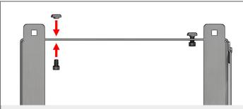
**Step 10.** Insert two *Cap Head Screws* from the bottom of the *Bracket* through the clearance holes and into two *Hammer Nuts*. Only start threading; leave loose for installation on the Festool MFT/3.
