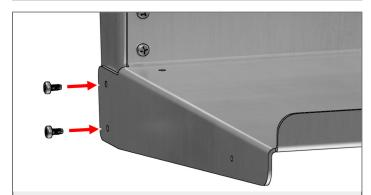
**Step 5.** Insert two more *Thread Forming Screws* through the *Base Pan* flange and into the *Bracket* legs. Repeat for the opposite side.
