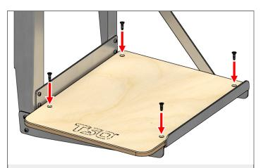
**Step 9.** Place the *Plywood Shelf* on the *Base Pan* with the TSO logo facing up and at the front of the shelf. Line up the holes in the *Plywood Shelf* and *Base Pan*. Insert four *Flathead Screws* through the *Plywood Shelf* and into the *Base Pan*.
