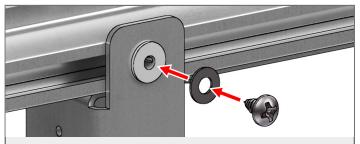
**Step 14.** Insert four *Phillips Round Head Screws* through the *Washers* and into the *Plastic Inserts*. Tighten by hand.
