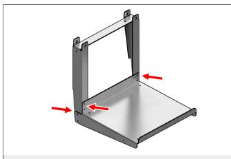
**Step 3.** Slide the *Bracket* down on the *Base Pan* as shown, so the *Bracket* legs fit inside the *Base Pan* flanges and the four holes on the *Base Pan* line up to the four holes in the *Bracket* legs.
