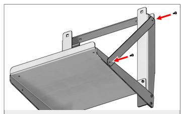
**Step 8.** Install *Shelf Brace* on the back side of the assembly using two *Thread Forming Screws* through the *Shelf Brace* and into the *Bracket* and *Base Pan*.
