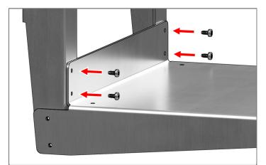
**Step 4.** Insert four *Thread Forming Screws* through the *Base Pan* and into the *Bracket* legs as shown. Do not tighten until Step 5 is complete.
