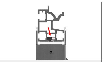
**Step 12.** Using a *5mm Hex Driver* or key, tighten both *Cap Screws* so the *Hammer Nuts* turn and clamp to the *MFT/3 Extrusion*, pulling the Tool Shelf up and tight.
