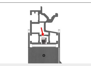
**Step 11.** Insert the Tool Shelf assembly into the *MFT/3 Extrusion* so the *Hammer Nuts* slide into the bottom T-slot and the *Bracket* flanges are on the outsides of the extrusion.
