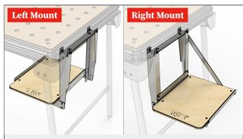
**Step 7.** Decide which way you plan to install your *MFT/3 Tool Shelf*, as this will determine its front and back. The remainder of this Assembly Guide will walk through installing it in the **Right Mount** configuration. If you prefer **Left Mount**, simply install the *Shelf Brace* on the opposite arm, and rotate the *Plywood Shelf* 180 degrees.
