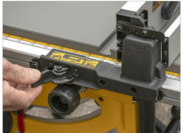
Step 1A. Unlock the fence levers located on the front and back of the DeWalt Fence Assembly .
