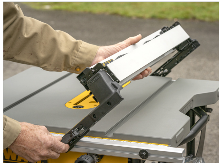
Step 1B. Lift the DeWalt Rip Fence off the table and place on an flat tabletop.
