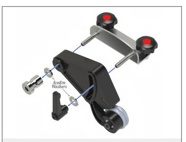
**STEP 2:** Insert the second bracket through the other JessEm stock guide body as shown. Secure by tightening JessEm handle and pivot knob. This guide will be located behind the table saw blade.
