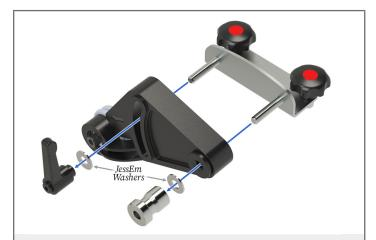
**STEP 1:** Insert bracket through the first JessEm stock guide body as shown. Secure by tightening the JessEm handle and pivot knob. This guide will be located forward of the table saw blade.
