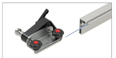
**STEP 3:** Slide both stock guides into the top T-track of the rip fence, observing the feed direction indicator arrow on the body of each JessEm stock guide. Once positioned, tighten both red star knobs securely. Follow the JessEm instructions to properly set the height of each stock guide to your workpiece.
