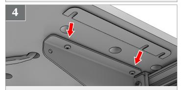
Insert *Spacers* between *Shelf Brackets* and the bottom of the *Tabletop*. Match the slots in the *Spacers* with the screw locations.
