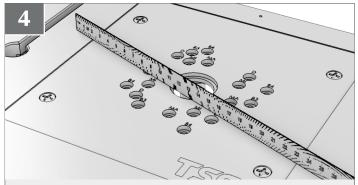
Confirm the Router Plate Insert is flush with the Router Table.
