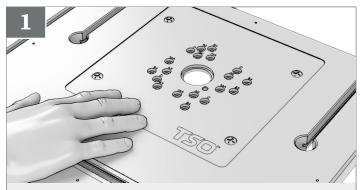
By finger feel or by using a straightedge (or using the included *Fence* as an alternative to a straightedge), determine if the Router Plate Insert is flush to the Router Table. If it is not, adjust by following these steps.
