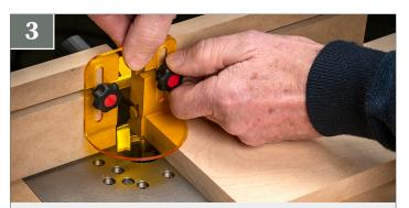
Adjust as needed and secure by tightening both *Small Knobs*. For the perfect fit, adjust your guard height to the workpiece as shown above.
