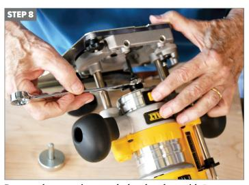
Remove the centering mandrel and replace with 5mm cutter (with 8mm shank), fully tightening the collet ready for use.
