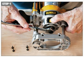
Remove DeWalt router base plate, saving the four phillips head screws. Replace the ¼" collett with 8mm collet using a 17mm open-end wrench included with your DeWalt router.
