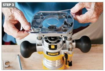
Orient the transparent TSO Adapter Plate as shown.
