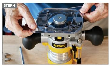
Attach TSO Adapter Plate by re-using the four (4) philips head screws, leaving them slightly loose.
