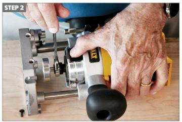
Insert Festool centering mandrel (with 8mm shaft) from LR 32 Set into 8mm collet and tighten.
