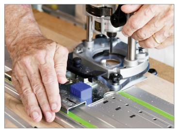
When not in use, store the TSO Pivot Block next to the Pivot Arm using it's magnetic base.
