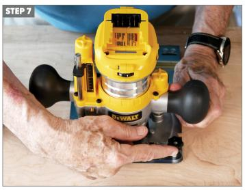
Flipping over the router, place both TSO Star Knobs on the threaded studs of the LR 32 Guide Plate and tighten.
