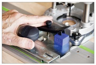
The TSO Pivot Block can be used to lock the Festool LR 32 Guide Plate pivot arm in the "up" position as shown when routing grooves, dados or rabbets.
