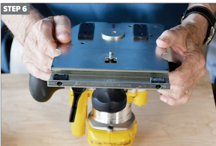
Place the Festool LR 32 Guide Plate on the router as shown, centering it over the mandrel.
