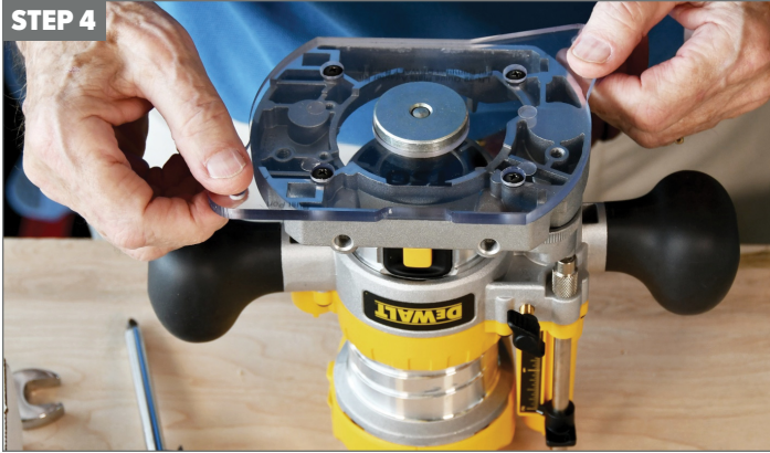
Attach TSO Adapter Plate by re-using the four (4) phillips head screws, leaving them slightly loose.
