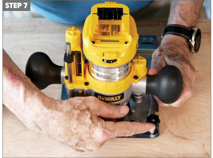
Flipping over the router, place both TSO Star Knobs on the threaded studs of the LR 32 Guide Plate and tighten.
