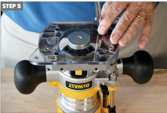
With the centering mandrel plunged through the TSO Adapter Plate, finish tightening the four (4) phillips head screws.
