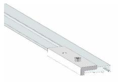
Clamp the fixture to assure that it won't move and drill through the hole using a 6-mm diameter or 15/64-inch diameter bit. Deburr the holes.
