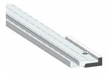
Fasten the drill fixture to the T-Track with the screw and nut provided with the screw oriented as shown above.
