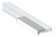
Clamp the drill fixture to the underside of the T-Track in the orientation shown with the end of the drill fixture flush with the end of the T-Track as shown above. Drill through both holes using a 6-mm diameter or 15/64-inch diameter bit. Deburr the holes.
