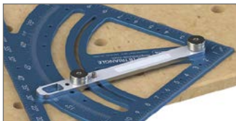
Step 3: Place Indexing Pointer on top of triangle and secure through worktop with both dogs
